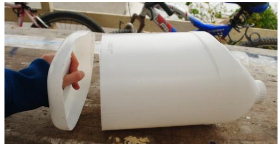
Össfass (correct spelling in Valerias opinion: Usfast) is a strange German word that means a device normally used to bail water out of a boat. However, you can also use it for collecting sediment from the seafloor and this is what we intended with our össfass-shaped device.
