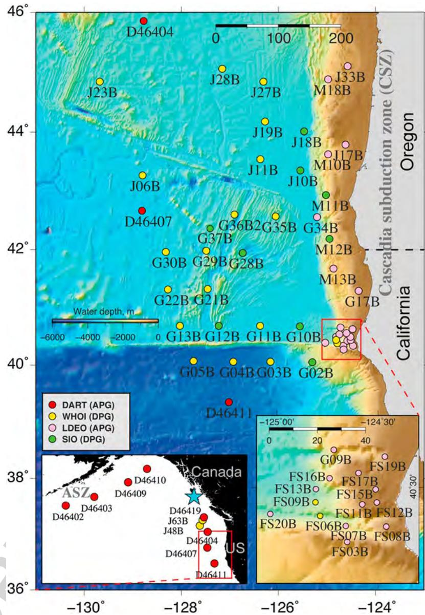
**Figure 1.** Station map of the tsunami dense array. Distribution of DART, APG, and DPG stations in the Cascadia (CSZ) and Aleutian subduction zones (ASZ). Light blue star represents the earthquake's epicenter.
