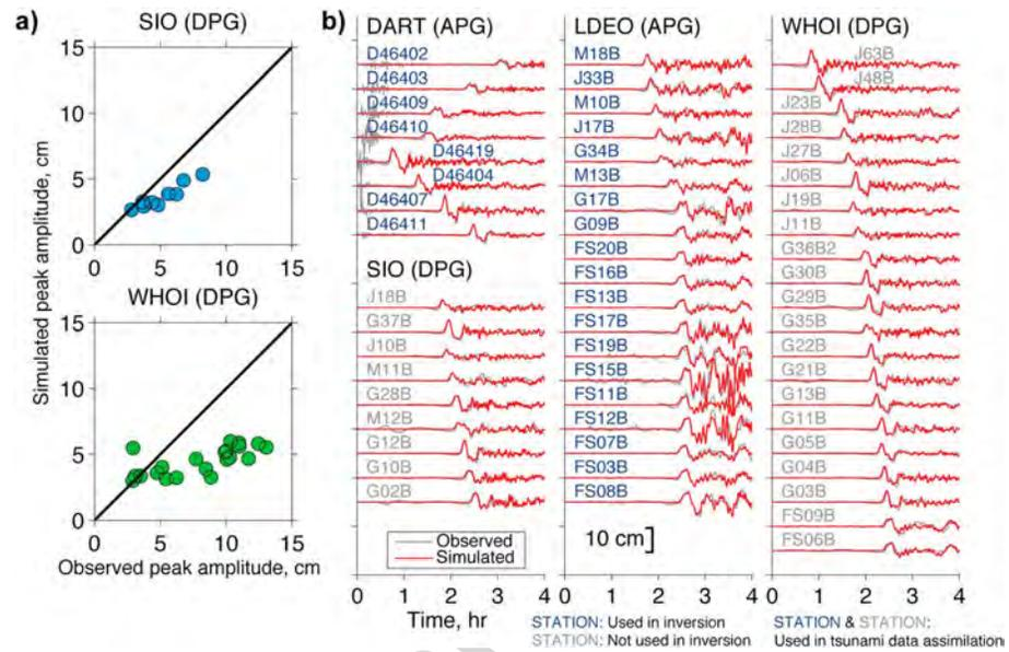
**Figure 2.** Tsunami simulation result. (a) Plots of simulated against observed peak amplitudes at SIO and WHOI stations. The ratios between the simulated and observed peak amplitudes are used for correction of DPG waveforms. (b) Comparison of observed/corrected (gray lines) and simulated tsunami waveforms from the estimated slip distribution (red lines). Station names at which tsunami waveforms are used in the inversion are written in blue.
